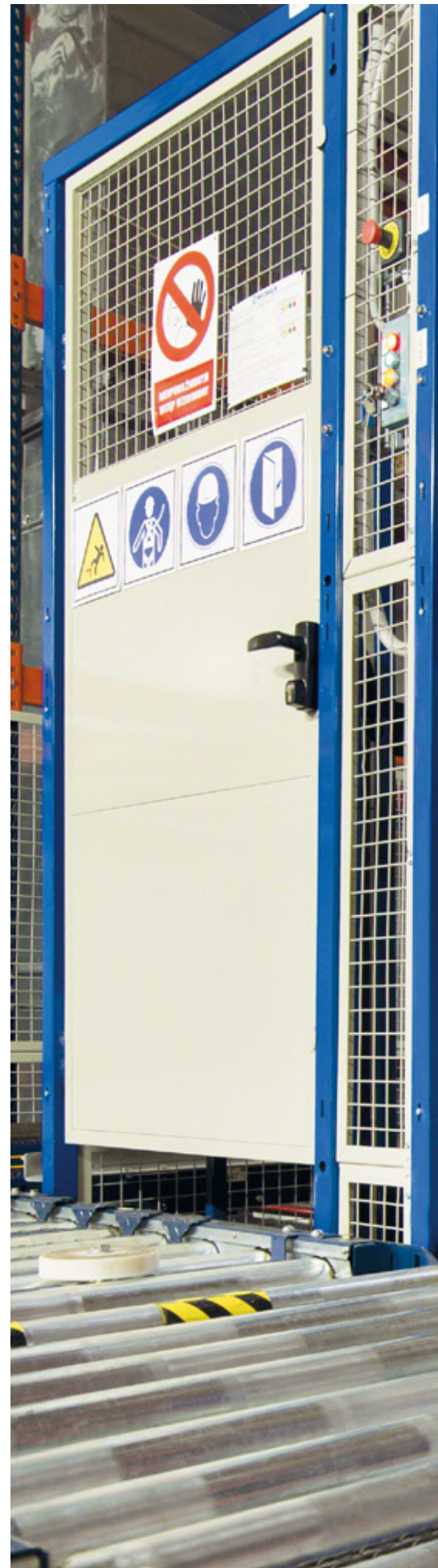
The mesh partitioning creates a protected space in the work zone that ensures operators are completely safe.
