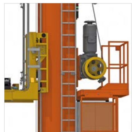
Hand ladder and top maintenance platform
